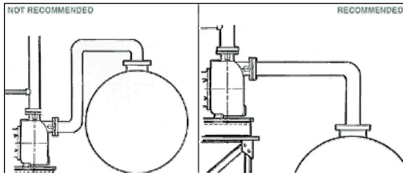
Fig. E Tank Car Unloading
